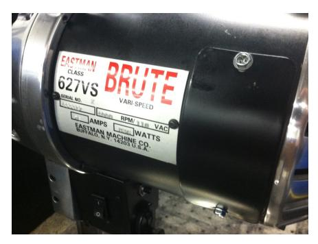
55. Tap two #4-40 holes on the motor for the name plate (79C1-159) to be attached with two #4-40  $\times$  1/8" screws (300C7-1).
