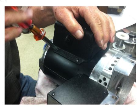
53. Remove the self-tapping threads from the four Thread Forming Screws (20C12-173). Place the speed control cover (53C11-158) on to the motor with the four screws.
