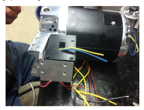
8. Install the switch base cover (53C5-237) with 3 screws (305C8-1) and feed the yellow and blue wires thru the switch opening and the two red w/black stripe wires out the other side of the front bearing housing.
