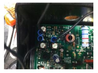
43. Connect these two wires to P2 and P3 on the speed control board as shown. And connect the only wire from the potentiometer with a blade connector to P1.
