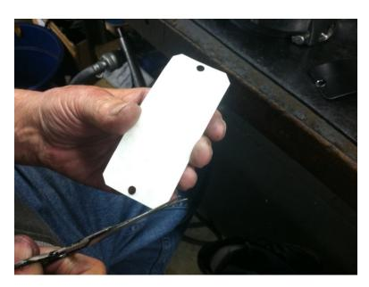
3. Trim down the brush insulator so that none of it is showing from behind the cover when fully assembled.
