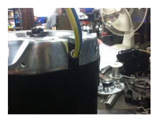
6. Place a piece of insulation on the blue and yellow wires that are coming out of the rear housing and push it down into the rear housing to prevent chafing of the wires.
