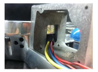
7. Place insulation over the four wires coming out of the front bearing housing and push it into the housing to prevent chafing of the wires.
