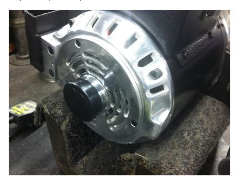
57. Assemble the Rear Cover (53C7-44) with the turning Knob (13C1-9), Spring (34C1-51), and Snap Ring (18C6-16)
