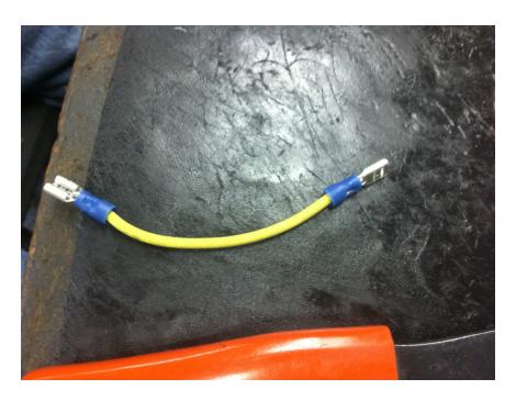
44. With a length of yellow wire roughly 3" strip both ends and attach two blade connectors as shown.
