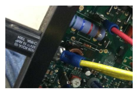
45. Insert the short yellow wire into the 10 amp circuit breaker (285C1-1) and the other end into L2 on the speed control board.
