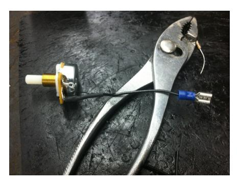
NOTE: Be sure to add a length of heat shrink to the wire before soldering.
