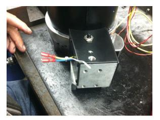
13. Strip the yellow and blue wires that are thru the switch opening and place a terminal end (47C4-79) on each wire. Zip tie (254C1) the two wires together as shown.
