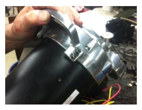
17. Attach the carrying handle (22C1-40) to the motor adaptor (29C6-165) with two #10-32  $\times$  5/8" screws (300C14-6).
