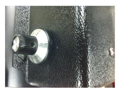
54. Install the Dial Indicator (104C1-6) onto the potentiometer and tighten the set screw, ensure that the "0" faces to the outside of the machine.
