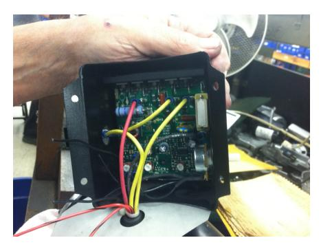
46. The two yellow wires from the motor body are to be connected to L1 on the speed control board and the other one to the Circuit Breaker. It does not matter which one goes where. Connect the red wire to A+ and the black wire to A- on the speed control board.
