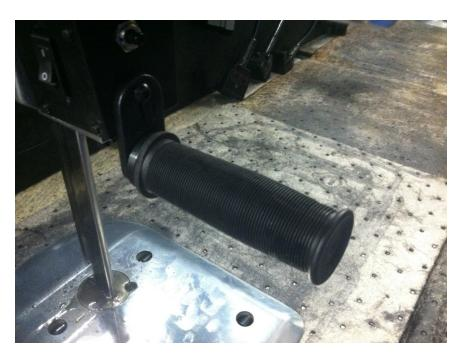
56. Install the Handle Bracket (62C1-140) with the Handle Bracket Screw (20C12-79) than install the Cushion Grip Handle (531C1-76) to the Handle Bracket.
