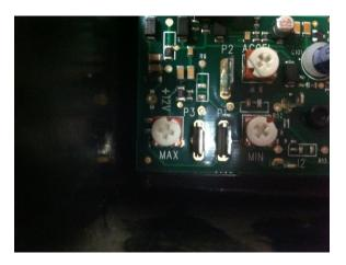
37. Set "ACCEL" to the 7 O'clock position and set "MAX" to the 1 O'clock position as shown.
