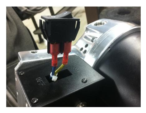
14. Connect the yellow and blue wires to the switch (580C1-198) as shown, and then push the switch into the switch cover.
