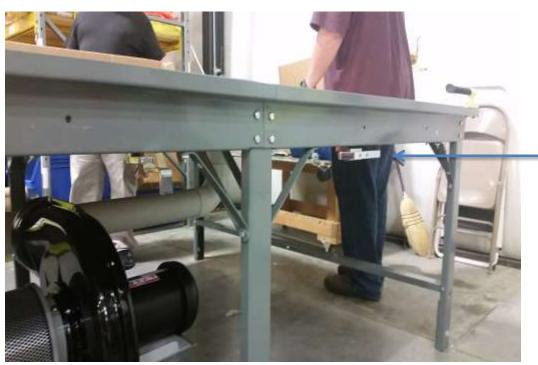
Attach the kill switch bracket to the operator side of the table.
