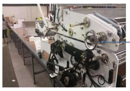
This wheel will need to be removed prior to putting on the top-cover on the non-operator side.
