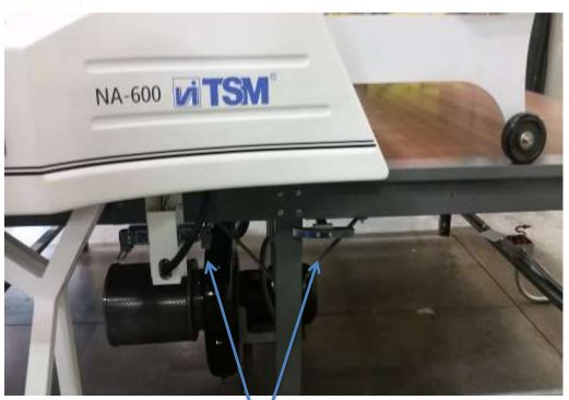
Now you can set the reversing sensor and the safety stop sensor along with the home sensor. Be sure you remember to tighten the bolts that were left loose at the beginning when you placed the switches down into place.
