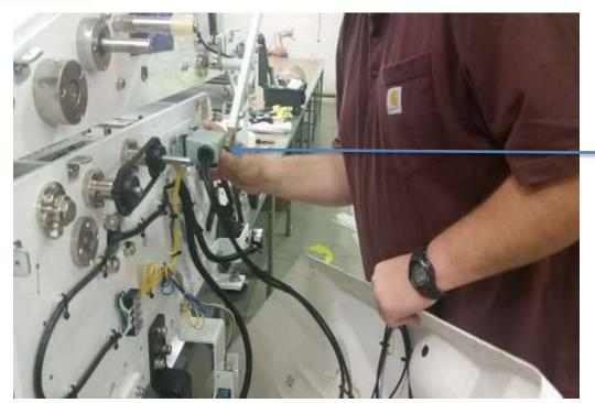
Take operator side cover and attached the male plug that is attached to the cover.
