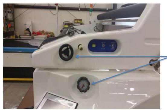
Attach manual-turn wheel on the operator side. Also, attach the tension control wheel to the machine.
