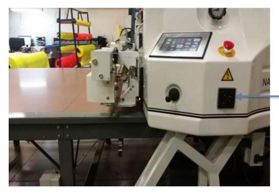
Then turn on the machine with the power switch. There will be a three second delay, than the machine will turn on.
