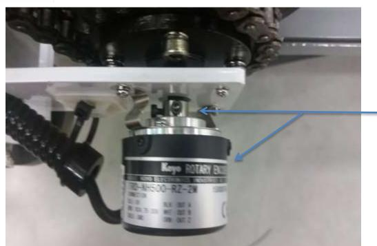
Make sure the setscrews are securely fastened with the encoder pushed all the way onto the rod.
