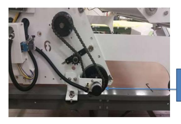
Attached the encoder to the bracket you just attached to the back table guided wheel.
