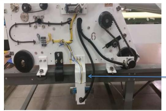
Loosen Bolts, than reverse the bracket that hold the limit switches. Wait to tighten these bolts until the safety and reversing switches are placed under the table at the end.
