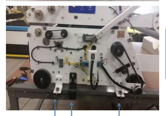
Here is an overall picture of the operator side. Attach the other Table guided wheel and bracket to the machine. Replicate on the non-operator side.
