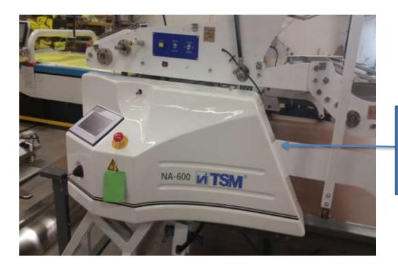
Attach the operator side cover to the
