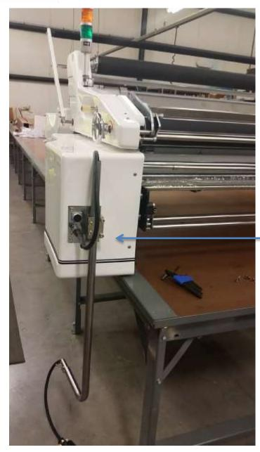
Attach the power pole to the machine. Plug it in.
