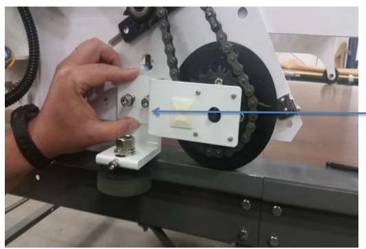
Attach the first table guided wheel to the table, than attach the white bracket seen here to the operator side back wheel.
