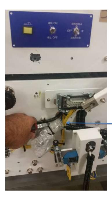
Snip Zip-tie on the encoder and remove the packaging from around the encoder.
