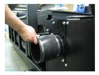
Insert the exhaust stack to the rubber boot.
