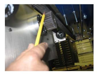
• Mount the E-chain trough to the frame on the non-operator side using (3) bolts.
