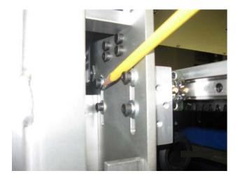
Adjust the back lash on the operator side and non operator side of the gantry using adjusting screws found on the back lash adjuster. Use a torpedo level to evenly raise the end plate and finally engage the spur gear into the rack and ensure there is no back lash.
