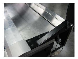
• Install the overlay tower to the finger end cap and secure the same with (5) screws. Repeat same procedure for non-operator side.
