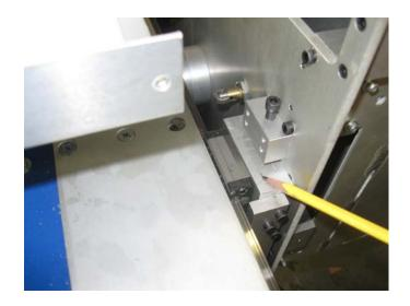
• Insert the screws to the bearing blocks so that it holds the bearings on the gantry.
