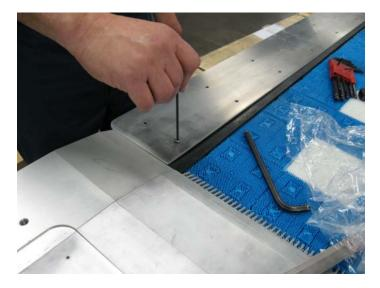
• Lay the dress plate on top of edge seal with the rounded corners facing outwards from the machine. Align the holes with the rack plate and edge seal. Install hardware, (30) pieces per dress plate. Repeat procedure on both sides of machine.
