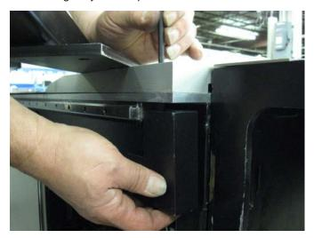
• Install the finger end caps at all four corners of the machine using the supplied hardware.
