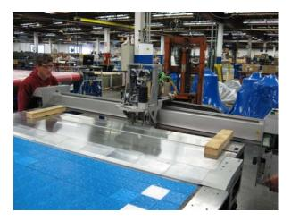
• Using two persons remove the gantry from the wooden crate and place it on the two stacks of wood on top of conveyor table.
