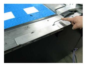
Install the gantry end stops at all four corners of the machine using the supplied hardware.
