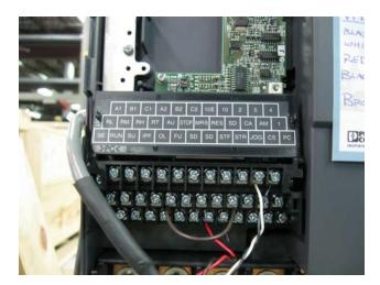
Flip the control wiring cover down.
