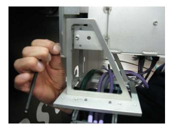
• Ensure that the gantry I/O, UIT cable, gantry out, gantry in, air line, power cable are connected to the non-operating side end plate.
