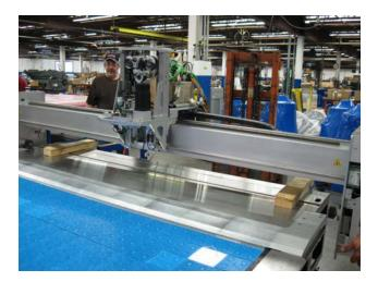
• Lift the gantry up and remove the wooden pieces, while holding the gantry in the same position drop it down to rest on the THK linear bearings, then slide the front bearings found on the take-on side both on the operator side and non-operator side.
