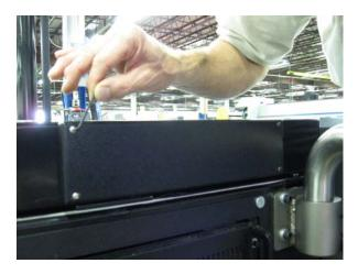
• Lay one end of transfer plate on the bristle fingers and the other end on the take-off conveyor, install (6) screws on the transfer plate to secure it to the bristle fingers.
