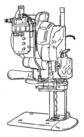
synthetic or plastic out of motor and sharpener twice a week. Remove the cover over cam. Clean and wipe off screw mechanism in sharpener once a week. Remove knife and clean knife slides with slot cleaner at least once a day. Clean and dry machine after any usage. To prevent undue accumulation, do not oil plate rollers. If rollers stick, remove from plate and wash in cleaning solvent.
