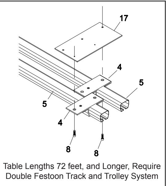
Table Lengths 72 feet, and Longer, Require Double Festoon Track and Trolley System
