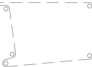
**EASIHOLD OVERLAY THREADING DIAGRAM**
