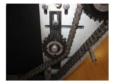
Put on the conveyor drive chain with master link around the sprockets.
