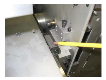
• Place the operator side THK linear bearing on the operator side rail facing towards the take-off side.
