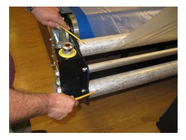
Mount the E-stops on both ends of the operator side.
