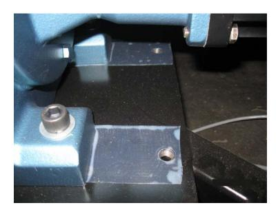
Loosen the split color and shaft color on the drive shaft.
