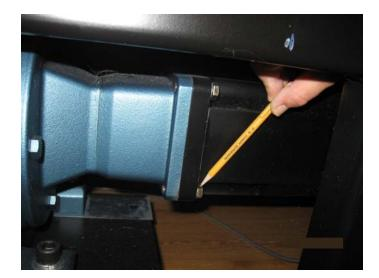
Plug the power cable and haul / encoder cable to the conveyor drive motor.
