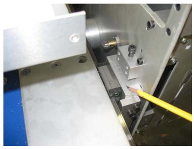
Insert the screws to the bearing blocks so that it holds the bearings on the gantry.
