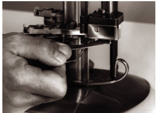
Figure 9. Adjusting Bevel Bloc Shoes
