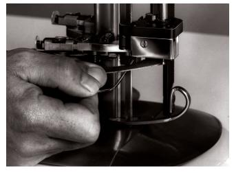
Figure 9. Adjusting Bevel Bloc Shoes
