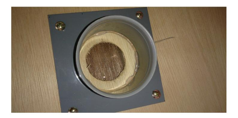
Smear glue around one head of L-shaped joint only and connect it to the bell mount
