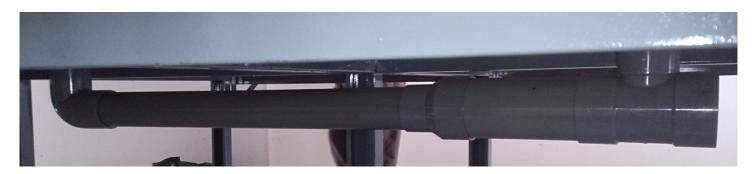
Smear glue around the head of T-shaped joint and connect with a short PVC pipe
